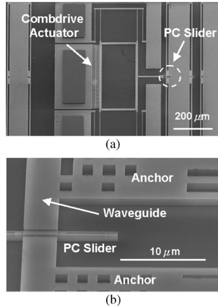
Fig. 3. (a) SEM image of fabricated MEMS PC switch. (b) Close-up view of PC slider. Two anchors support suspended waveguides.
