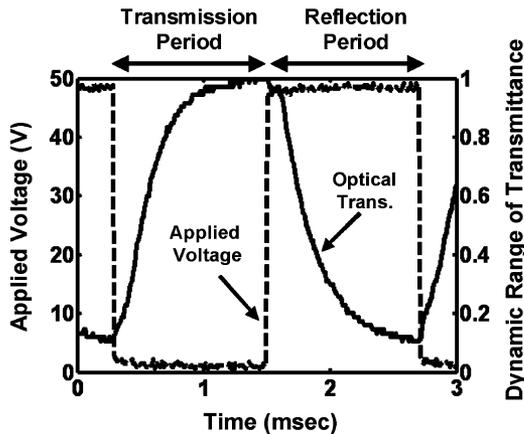
Fig. 5. Measured dynamic response of switch. Applied voltage is a square wave with period of 2.5 ms (dashed curve). Optical signal is measured by photodetector (solid curve).
