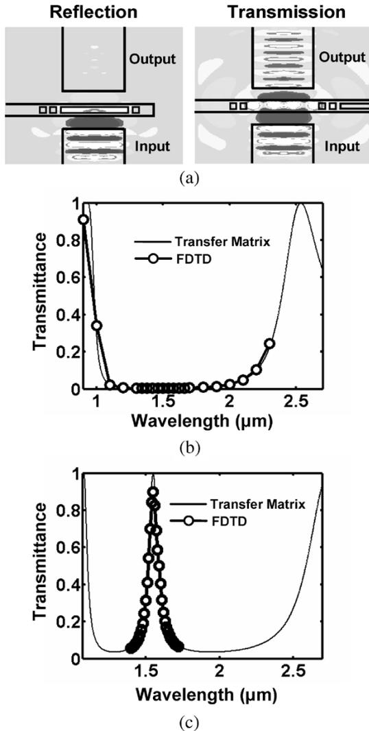
Fig. 2. (a) 2-D FDTD simulation at transmission state and reflection state. Calculated transmission spectra for (a) transmission state and (b) reflection state.
