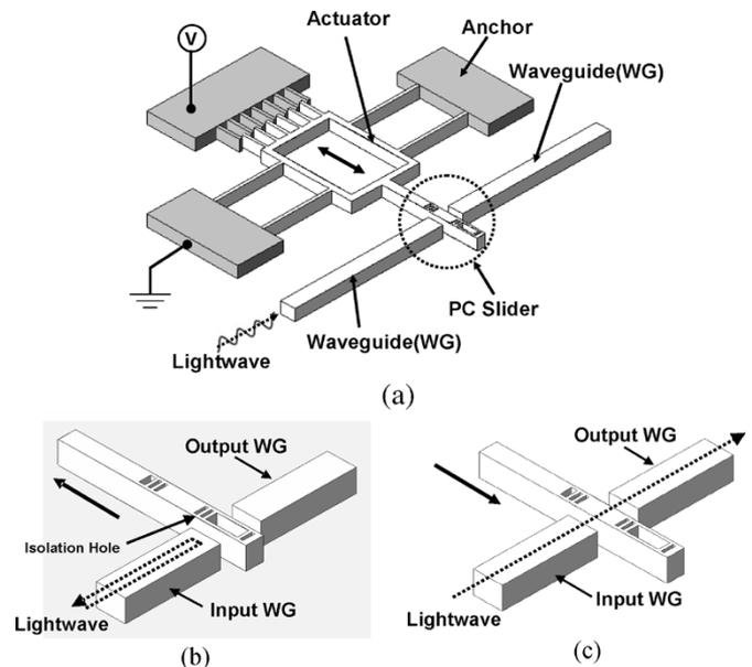
Fig. 1. (a) Schematic of MEMS-actuated PC switch. Lateral comb-drive actuator connects with PC slider inserted between two waveguides. Two states are defined on tip of PC slider: (b) reflection state and (c) transmission state.
