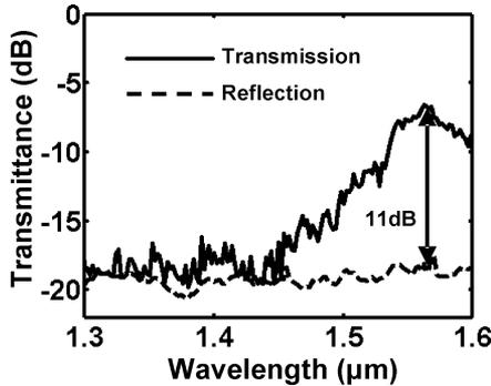
Fig. 4. Measured optical spectra at transmission (solid curve) and reflection states (dashed curve).
